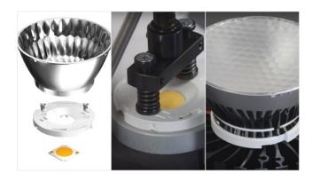
BJB LED Holders (47.319 Series) enable simple assembly of components for spot and downlights applications. The holders feature COB pre-fixation clips which provide secure retention of the LED array while mounting to a heatsink. And with a standardized reflector interface, BJB reflectors (in addition to reflector solutions from ecosystem partners) can be easily mated to the holder - simply twist-and-lock into place.
