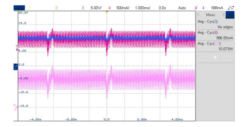
The below plot represents the measured current through the LEDs when the LEDs are at 65° C:
