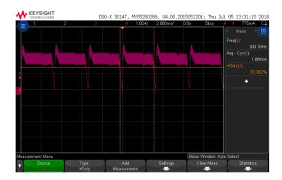
The below plot represents the measured current through the LEDs when the LEDs are at 73° C:
