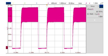
The below plot represents the measured current through the LEDs when the LEDs are 80° C:
