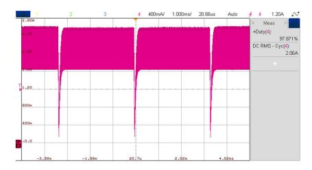
The below plot represents the measured current through the LEDs when the LEDs are at 76° C:
