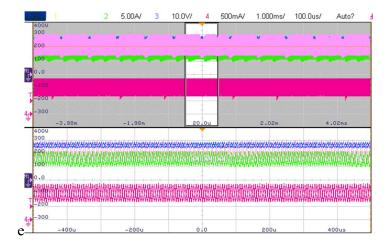
The below plot represents the measured current through the LEDs when the LEDs are at 55° C:
