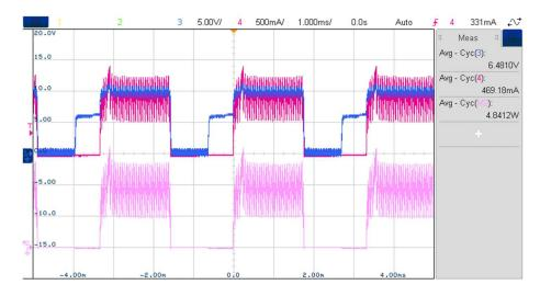
As shown, the current pulse width is lowered, thus lowering the average current through the LEDs, as the temperature increases.
