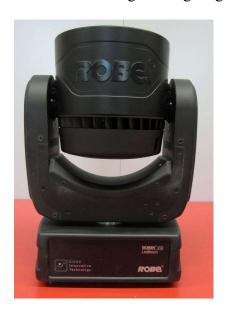
155. On information and belief, LEDBeam 150 products include a LED module mechanically enclosed by the lighting fixture; for example, an LED module, comprising LEDs, an LED driver, and a thermal sensor is mechanically enclosed by the housing.
