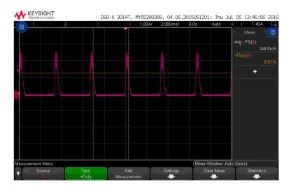
As shown, the current pulse width is lowered, thus lowering the average current through the LEDs, as the temperature increases.
