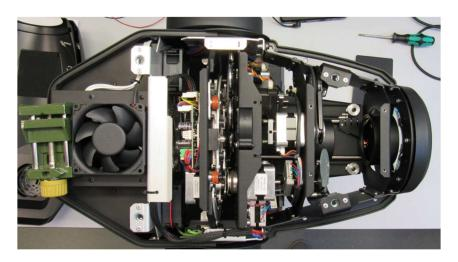
144. On information and belief, the LED module includes at least one LED; for example, the LED module includes a 480 Watt RGBW LED engine including LEDs arranged into sixteen LED strings.
