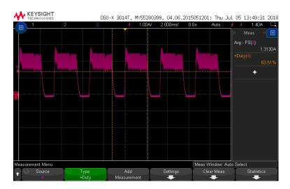
The below plot represents the measured current through the LEDs when the LEDs are at 88° C:
