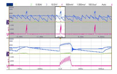
As shown, the current pulse width is lowered, thus lowering the average current through the LEDs, as the temperature increases.
