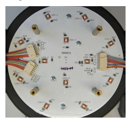
163. On information and belief, the LED module includes a LED driver in electrical communication with the at least one LED to operably provide a LED drive signal to the at least one LED; for example, LEDBeam 100 products contain an LED driver in electrical communication with the twelve LED strings to operably provide a respective LED drive signals to each of the LED strings.
