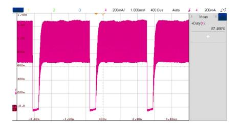
The below plot represents the measured current through the LEDs when the LEDs are at 87° C:
