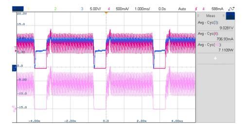
The below plot represents the measured current through the LEDs when the LEDs are 70° C:
