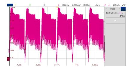
The below plot represents the measured current through the LEDs when the LEDs are at  $75^{\circ}$  C:
