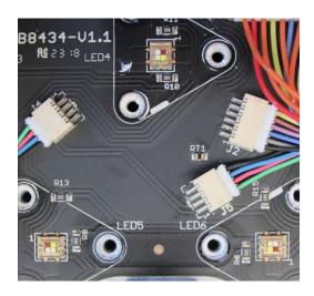
157. On information and belief, the LED module includes a LED driver in electrical communication with the at least one LED to operably provide a LED drive signal to the at least one LED; for example, LEDBeam 150 products contain an LED driver in electrical communication with the four LED strings to operably provide a respective LED drive signals to each of the LED strings.
