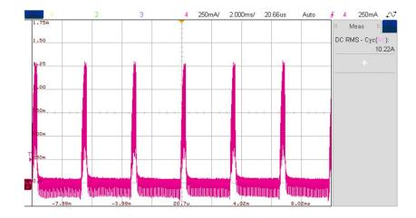
As shown, the current pulse width is lowered, thus lowering the average current through the LEDs, as the temperature increases.
