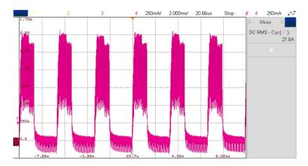
The below plot represents the measured current through the LEDs when the LEDs are 80° C:
