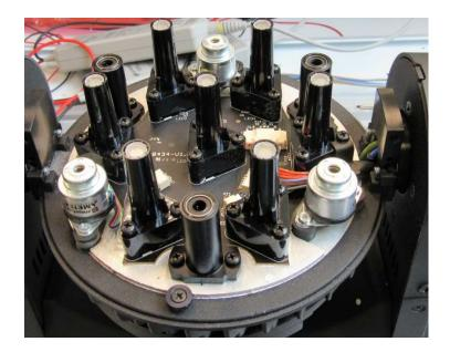
189. On information and belief, each light source has a second reference axis indicating an orientation of the light source, the second reference axis for each light source being designated identically for all light sources of the plurality of light sources; for example, each RGBW multichip has a second reference axis taken through the center of the RGBW multichip, parallel to the longer side of the multichip's rectangular shape.
