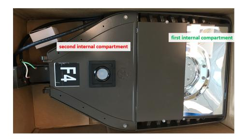
102. The first internal compartment of the Evolve LED Area Light EALS contains one or more light emitting diodes (elements), as shown in the pictures above and below, that are mounted on a base connected to the housing.
