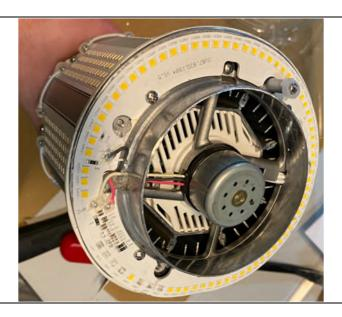
123. The GE LED HID Replacement contains a driver that is spatially separated from and configured for powering said light source as shown in the picture below:
