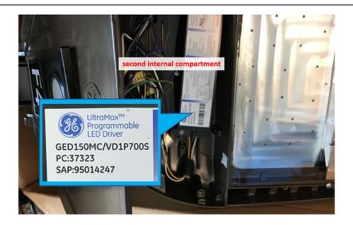
104. On information and belief, the Evolve LED Area Light EALS's first internal compartment is thermally separated from the second internal compartment, each of said first internal compartment and said second internal compartment configured to dissipate heat.
