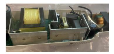
126. Upon information and belief, the GE LED HID Replacement's light source heat sink and the driver heat sink are separated by an air gap to provide thermal decoupling of the light
